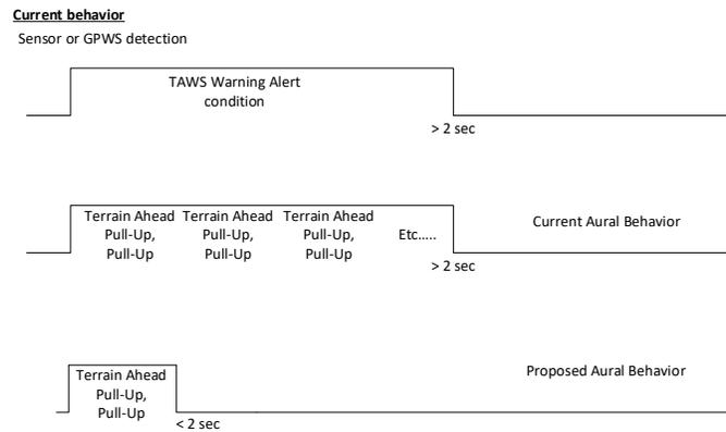
**Figure A-7: Block Diagram of Current and Proposed Aural Behavior**
